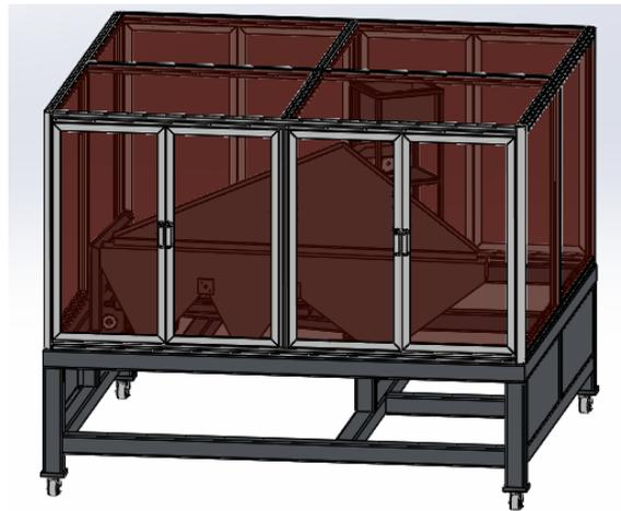
Fig. 2. Experimental equipment for vibration separation
